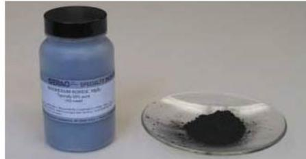
Figure 1 | The newly discovered superconductor magnesium boride has been available in large quantities from suppliers of inorganic chemicals for many years, but physicists have finally bubbled the champagne and found that magnesium boride superconducts at an amazing 39 K (ref. 1).
