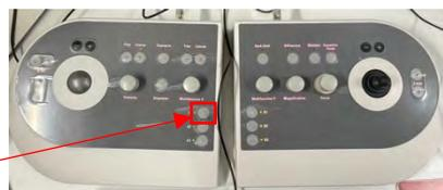
The  $\alpha$  wobbler of the L1 control board is also enabled.
