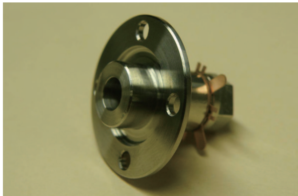
Figure caption: Transducer of piezoelectric actuator for cryogenic temperature.
