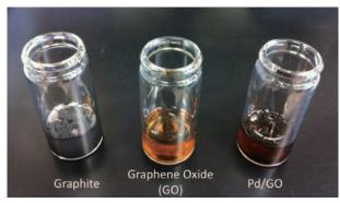
Fig. 2. Pictures of insoluble graphite (left), aqueous solution of GO (middle), and aqueous solution of Pd/GO composite.
