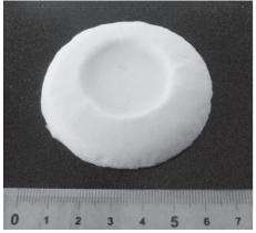
Fig. 3. Photograph of as-prepared larger ZSM-5 bulk bodies.
