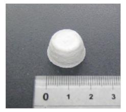
Fig.1. Photograph of as-prepared ZSM-5 bulk bodies.
