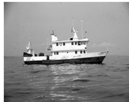
R/V TANGANYIKA EXPLORER, chartered vessel for the LTR; two masts for a weather station on the roof; the ship ADCP was installed on the starboard side next to the open gate.
