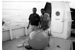
Buoy based on ACDP ready for deployment
