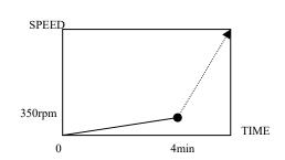
At the ACCEL 5 setting, it will change into the maximum acceleration in 4min. At the DECEL 5 setting, it takes 4min from 350 to 0 rpm after it decelerates by the maximum deceleration.
